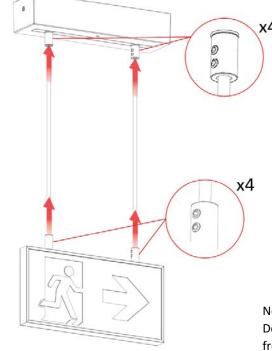
Note: Rods can be cut to desired length (if required). Debur cut ends and remove any coating 10-12mm from rod end to provide electrical connection
